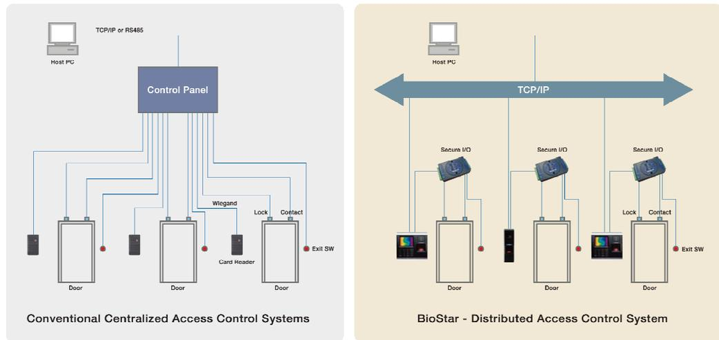
BioStar is a server-client application that supports up to 32 clients (2 clients maximum in the free version). A typical configuration consists of numerous access control devices connected to a central server via Ethernet, WLAN, and/or RS485. BioStar is compatible with MS SQL Server and MySQL databases.
